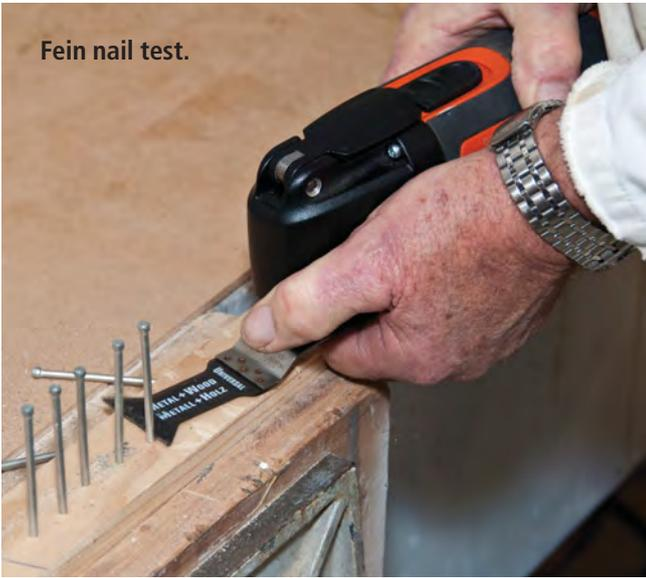
frame. Builders often use reciprocating tools for this job but multi-cutters can do it without damaging the timber of the door or window surround. That's what the bimetal blade is designed for, to be able to cut through timber with nails. In the nail test we measured the time the tool took to cut through ten 90 mm x 2.5 mm nails typically used in framing.
