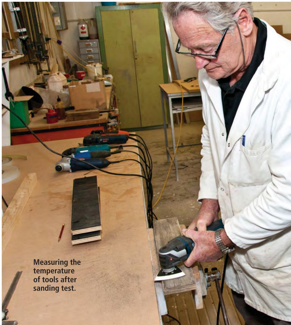
**Measuring the temperature of tools after sanding test.**
